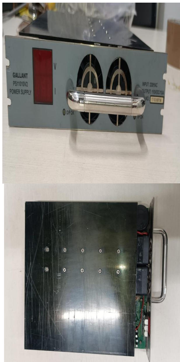
Fig. 13 Power Supply Unit 230V AC/110V DC
