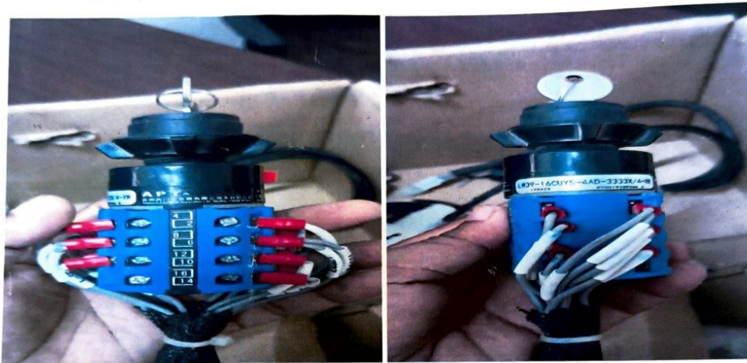
4. LCB ASD (Rotary Selection switch 4 position with key) (part no. LW39-16CUYS-4AD-3333X/4-XW)
