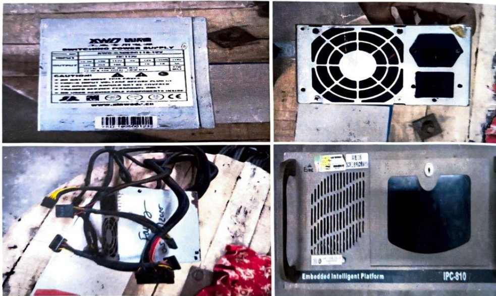
2. SMPS for CPU (I/P 110V DC, O/P +3.3V, +5V, +12V, -12V, +5VSB), 350 watt
